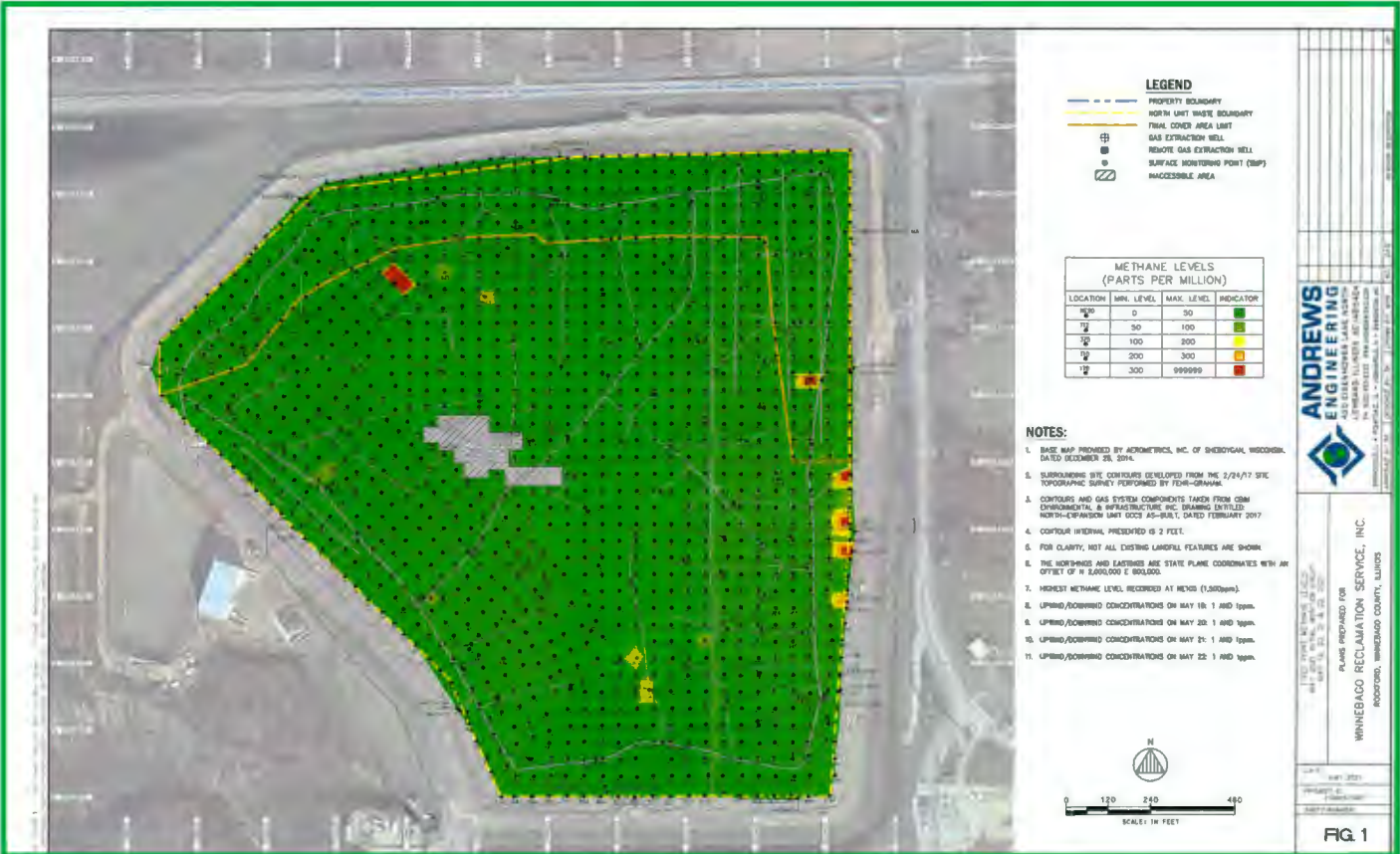
May 2021 status report filed by Waste Connections Winnebago Landfill operator in Rockford, Illinois reported 5 exceedances over 300 ppm in the Northern Expansion Unit. Image Credit: EPA Inspection Report
