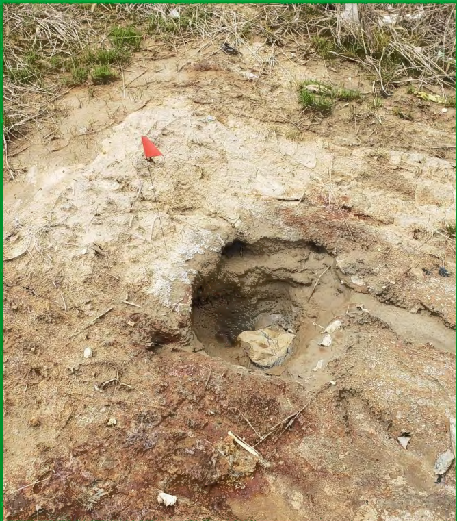
Photo of a SEM exceedance with audible bubbling liquid, Prairie Hill Landfill, Morrison, Illinois Image credit: EPA Inspection Report
