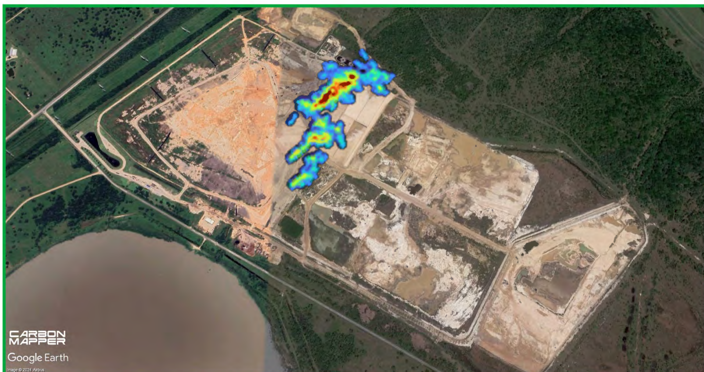
Methane plume observed by Carbon Mapper during aerial monitoring at a landfill in Texas Image Credit: Carbon Mapper
